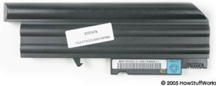
Figure 2 - Example of a Lithium Ion Battery Transport as Cargo
